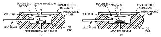
Figure 4. Cross-Sectional Diagrams (Not to Scale)
