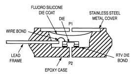
Figure 3. Cross–Sectional Diagram (Not to Scale)
