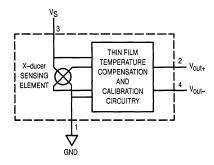
Figure 1. Temperature Compensated Pressure Sensor Schematic
