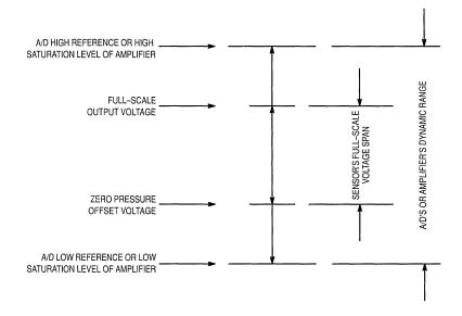
Figure 1. Positioning the Sensor's Full-Scale Span within the A/D's or Amplifier's Dynamic Range
