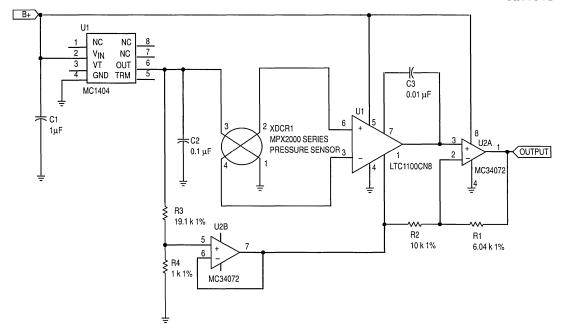
Figure 3. Precision Instrument Amplifier Interface
