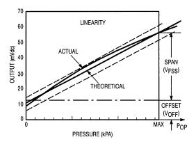
Figure 2. Linearity Specification Comparison
