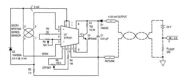
Figure 9. 4-20 mA Pressure Transducer
