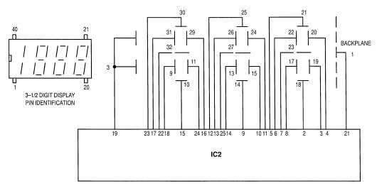
Figure 4. IC2 Driving Optional 3-1/2 Digit LCD Display
