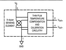
Figure 1. Temperature Compensated Pressure Sensor Schematic
