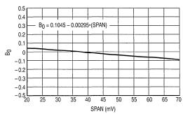
Figure 3. MPX10 Linearity Analysis — Correlation of  $B_0 V_{Out} = B_0 + B_1 (P) + B_2 (P)^2$
