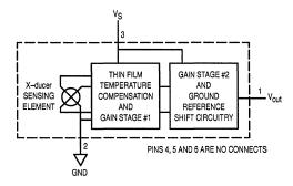
Figure 1. Fully Integrated Pressure Sensor Schematic
