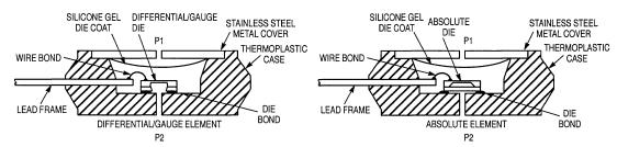
Figure 4. Cross-Sectional Diagrams (Not to Scale)
