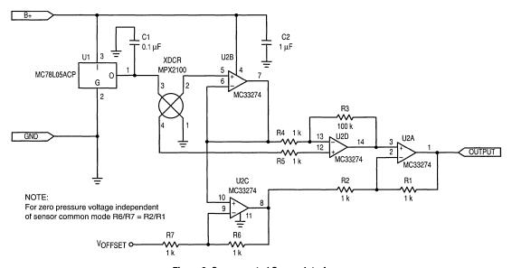
Figure 3. Compensated Sensor Interface
