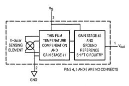
Figure 1. Fully Integrated Pressure Sensor Schematic
