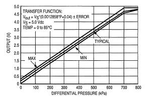
Figure 2. Output versus Pressure Differential
