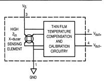
Figure 1. Temperature Compensated Pressure Sensor Schematic
