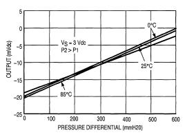
Figure 2. Output versus Pressure Differential
