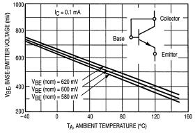
Figure 1. Base-Emitter Voltage versus Ambient Temperature
