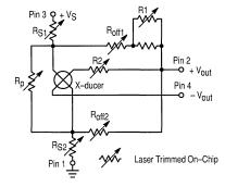
Figure 1. Pressure Sensor MPX2000 Series
