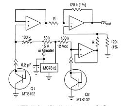
NOTE: With Q1 and Q2 at identical temperature, adjust R<sub>CAL</sub> for V<sub>Out</sub> = 0.000 V  $R = 15 \ k\Omega \ (1\%) \ for \ ^oF$
