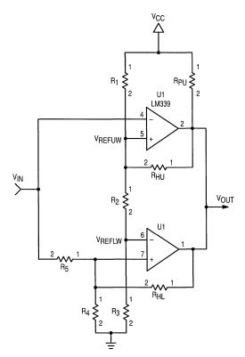
Figure 9. The LM339 Window Comparator Circuit
