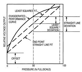
Figure 2. Linearity Specification Comparison
