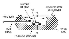
Figure 3. Cross–Sectional Diagram (Not to Scale)
