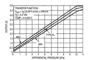
Figure 4. Output versus Pressure Differential
