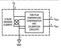
Figure 1. Temperature Compensated Pressure Sensor Schematic
