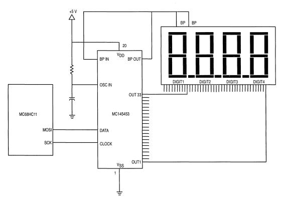
Figure 4. LCD Display Interface Diagram
