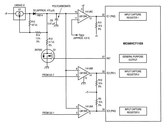
Figure 3. Analog-to-Digital Converter Front End with Microcontroller
