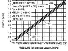
Figure 3. Output versus Absolute Pressure
