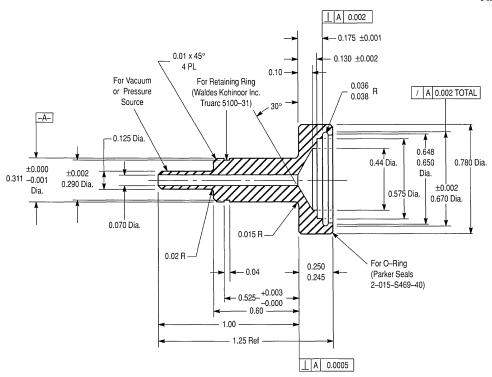
Figure 8. O-Ring Test Fixture
