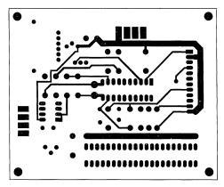
Figure 9. PCB Solder Side Artwork
