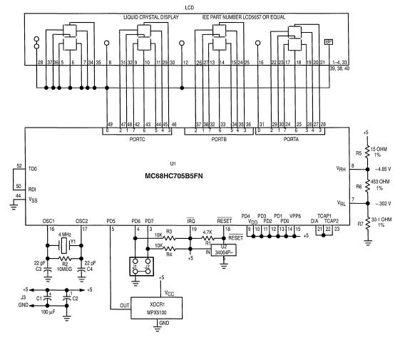
Figure 2. DEVB-114 System Schematic
