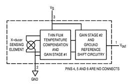
Figure 1. Fully Integrated Pressure Sensor Schematic
