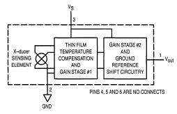
Figure 1. Fully Integrated Pressure Sensor Schematic
