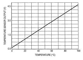
Figure 4. Temperature Sensor Output versus Temperature
