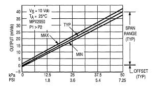
Figure 3. Output versus Pressure Differential
