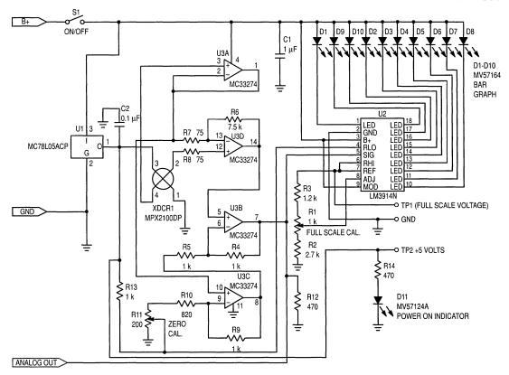
Figure 2. Compensated Pressure Sensor EVB Schematic
