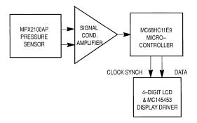
Figure 2. Barometer System Block Diagram
