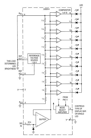
Figure 4. LM3914 Block Diagram
