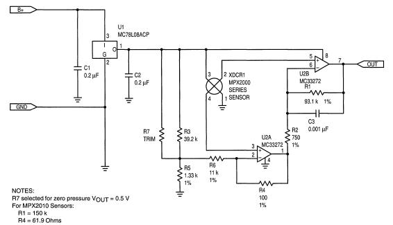
Figure 2. Sensor Mini Block
