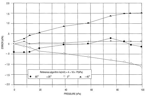
Reference algorithm is the straight from output at 255 0 pressure and output at full pressure
