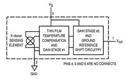
Figure 1. Fully Integrated Pressure Sensor Schematic
