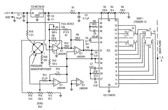
Figure 3. Schematic Diagram of Digital Pressure Gauge
