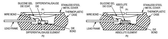
Figure 4. Cross-Sectional Diagrams (Not to Scale)
