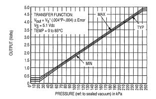
Figure 4. Output versus Absolute Pressure
