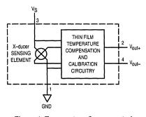
Figure 1. Temperature Compensated Pressure Sensor Schematic
