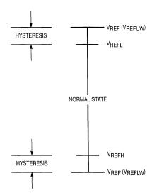
Figure 6. Setting the Reference Voltages
