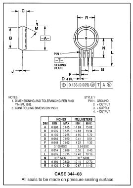
Figure 6. Chip-Carrier Package
