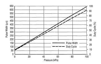
Figure 6. PWM Output Pressure Sensor Linearity Data
