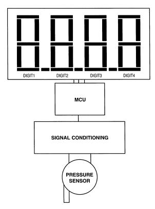
Figure 1. Barometer System
