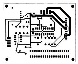
Figure 8. PCB Component Side Artwork
