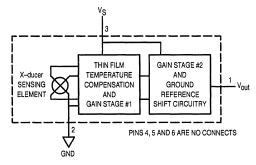
Figure 1. Fully Integrated Pressure Sensor Schematic
