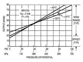
Figure 2. Output versus Pressure Differential
