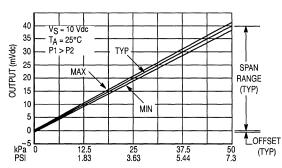
Figure 3. Output versus Pressure Differential
