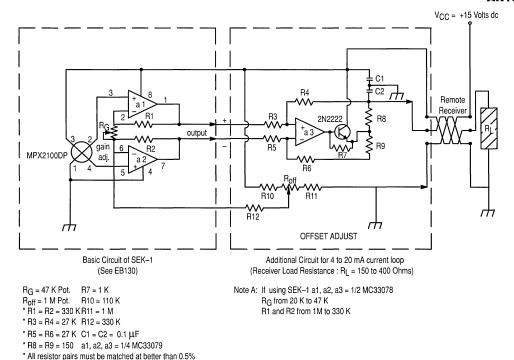
NOTICE: THE PRESSURE SENSOR OUTPUT IS RATIOMETRIC TO THE POWER SUPPLY VOLTAGE. THE OUTPUT WILL CHANGE WITH THE SAME RATIO AS VOLTAGE CHANGE.
