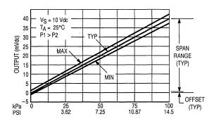
Figure 3. Output versus Pressure Differential
