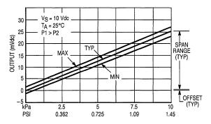
Figure 2. Output versus Pressure Differential
