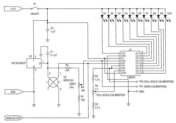
Figure 2. MPX5100 Pressure Gauge
