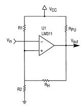
Figure 2. LM311 Comparator Circuit Schematic
