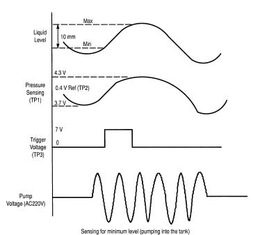
The sensing probe is tied to the positive pressure port of the sensor. The pump is turned on to fill the tank when the minimum level is reached.
