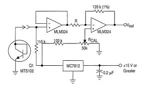
NOTE: With Q1 at a known temperature, adjust R<sub>CAL</sub> to set output voltage to  $V_{out}$  = TEMP x 10 mV, Output of MTS102, 3, 5 is then converted to  $V_{out}$  = 10 mV/° – (°F, °C or °K)
