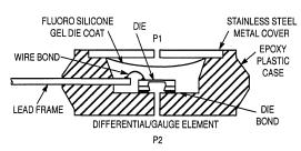
Figure 3. Cross–Sectional Diagram (Not to Scale)
