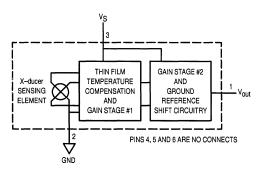
Figure 1. Fully Integrated Pressure Sensor Schematic
