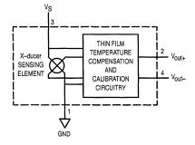
Figure 1. Temperature Compensated Pressure Sensor Schematic
