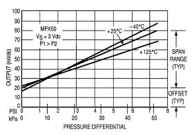
Figure 2. Output versus Pressure Differential
