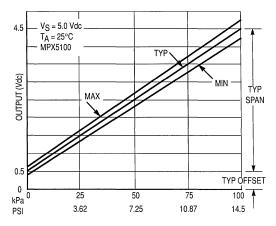
Figure 4. MPX5100 Output versus Pressure Input
