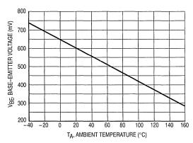
Figure 3. VBE versus Ambient Temperature Characteristic
