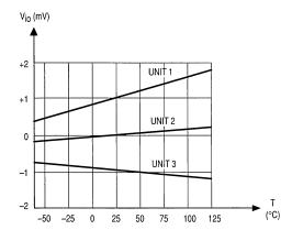
Figure 6. Input Offset Voltage versus Temperature
