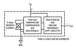
Figure 1. Fully Integrated Pressure Sensor Schematic
