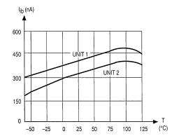
Figure 7. Input Bias Current versus Temperature
