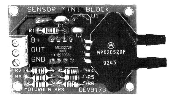
Figure 1. DEVB173 Sensor Building Block Evaluation Board
