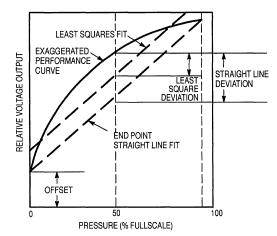
Figure 4. Linearity Specification Comparison
