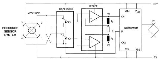
Figure 9. Two Channel Input and One Output Port Are Used by the MCU
