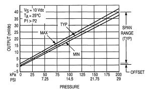
Figure 3. Output versus Pressure Differential
