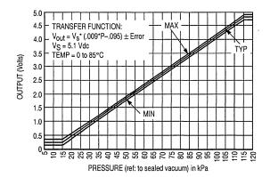
Figure 4. Output versus Absolute Pressure
