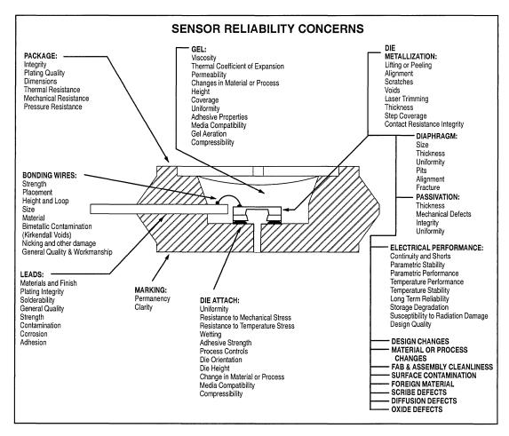
Figure 10. Process and Product Variability Concerns During Reliability Testing
