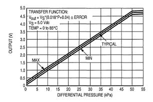
Figure 2. Output versus Pressure Differential
