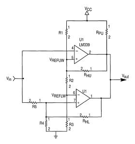
Figure 6. LM339 Window Comparator Circuit Schematic
