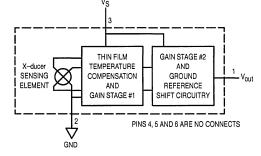
Figure 1. Fully Integrated Pressure Sensor Schematic
