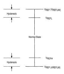
Figure 3. Setting the Reference Voltages
