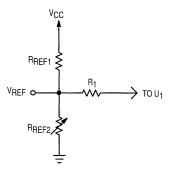
Figure 3. A Resistor Divider to Create VREF
