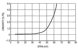
Figure 2. MPX10 Series Span versus Linearity
