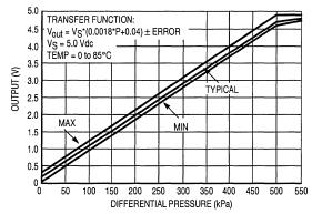
Figure 2. Output versus Pressure Differential
