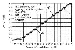
Figure 4. Output versus Absolute Pressure
