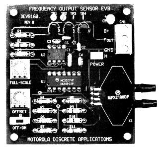
Figure 1. DEVB160 Frequency Output Sensor EVB
