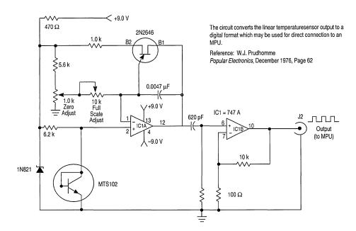
All resistors are 10% 1/4 watt except 6.2 k which is 5% 1/4 watt.
