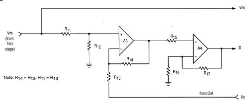
Figure 4. Second Stage — Difference Amplifier and Gain
