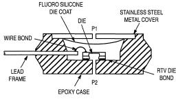
Figure 3. Cross–Sectional Diagram (Not to Scale)
