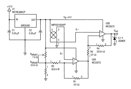
Figure 3. Signal Conditioning Circuit
