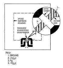
Figure 1. Basic Uncompensated Sensor Element — Top View
