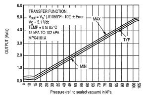
Figure 5. Output versus Absolute Pressure
