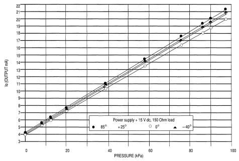
Figure 2. Output versus Pressure
