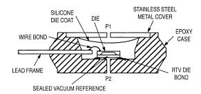
Figure 2. Cross–Sectional Diagram (Not to Scale)
