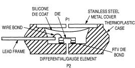
Figure 4. Cross–Sectional Diagram (not to scale)
