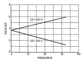
Figure 2. Instrument Amplifier Transfer Function
