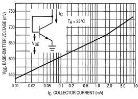
Figure 2. Base–Emitter Voltage versus Collector–Emitter Current
