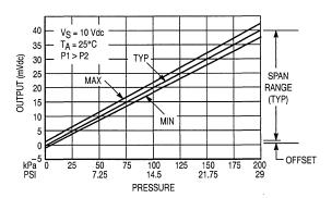
Figure 3. Output versus Pressure Differential
