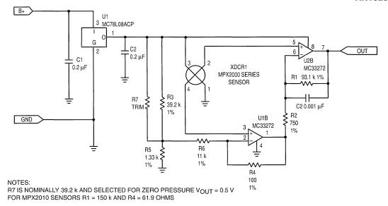
Figure 4. Sensor Mini Amp
