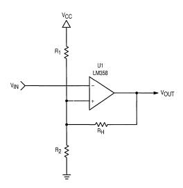
Figure 7. The LM358 Comparator Circuit Schematic
