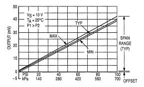
Figure 3. Output versus Pressure Differential
