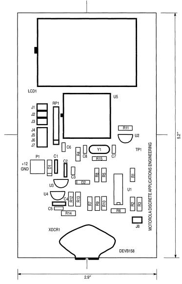
Figure 2. Printed Circuit Silkscreen
