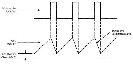
Figure 2. Ideal Ramp Waveform for the PWM Output Pressure Sensor
