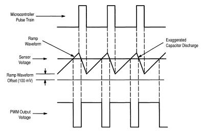
Figure 5. Relationships Between the PWM Output Pressure Sensor Voltages
