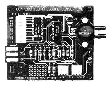
Figure 1. DEVB147 Compensated Pressure Sensor Evaluation Board
