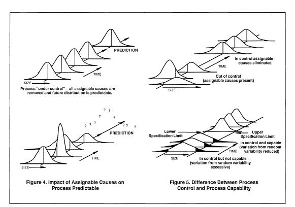
At Motorola, for critical parameters, the process capability is acceptable with a Cpk = 1.33. The desired process capability is a Cpk = 2 and the ideal is a Cpk = 5. Cpk, by definition, shows where the current production process fits with relationship to the specification limits. Off center distributions or excessive process variability will result in less than optimum conditions
