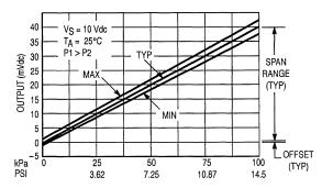
Figure 3. Output versus Pressure Differential
