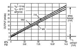
Linearity of output and less than  $\pm 1$  mV variation in Offset over a temperature range from -40 to  $125^{\circ}C$  attest to the excellent performance of the compensated series of MPX pressure sensors.
