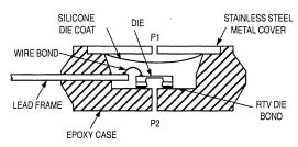
Figure 2. Cross–Sectional Diagram (Not to Scale)
