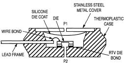
Figure 3. Cross-Sectional Diagram (not to scale)
