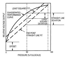
Figure 2. Linearity Specification Comparison
