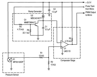
Figure 1. PWM Output Pressure Sensor Schematic
