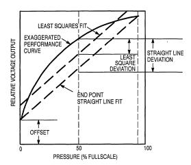
Figure 2. Linearity Specification Comparison
