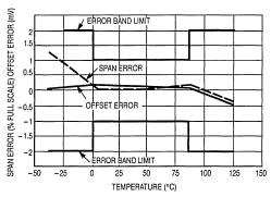
Curves of span and offset errors indicate the accuracy resulting from on-chip compensation and laser trimming.
