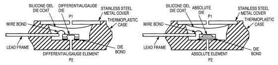
Figure 4. Cross-Sectional Diagrams (Not to Scale)
