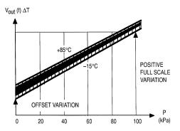
Figure 3. Output Voltage versus Temperature. The Dark Area Shows the Trend of the Compensation
