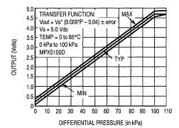
Figure 4. Output versus Pressure Differential
