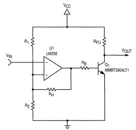
Figure 8. The LM358 with a Transistor Output Stage Comparator Circuit
