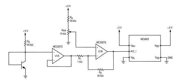
Figure 2. Analog Temperature Sensing Circuit
