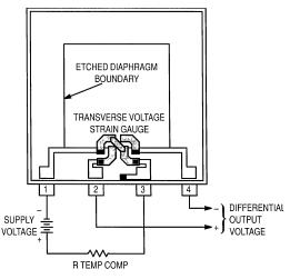
Figure 1. Sensor Construction Showing Electrical Connections
