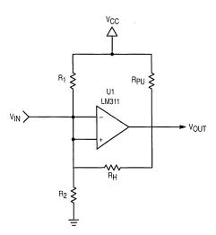
Figure 5. The LM311 Comparator Circuit Schematic
