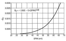
Figure 5. MPX10 Linearity Analysis — Correlation of  $B_2 V_{out} = B_0 + B_1 (P) + B_2 (P)^2$
