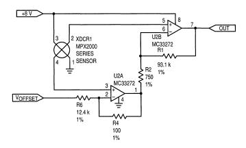
Figure 3. Simplified Schematic
