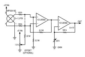
**Microprocessor Interface Circuit**
