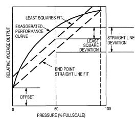
Figure 2. Linearity Specification Comparison
