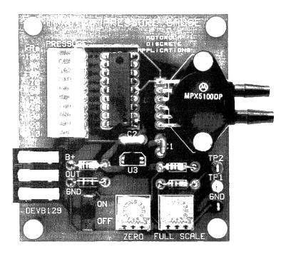
Figure 1. DEVB129 MPX5100 Bar Graph Pressure Gauge
