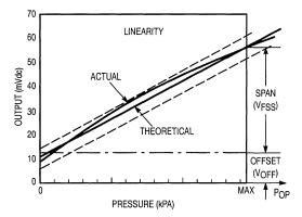
Figure 3. Linearity Specification Comparison
