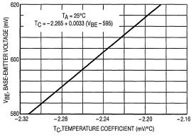
Figure 3. Temperature Coefficient versus Base–Emitter Voltage
