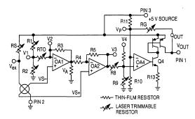
**Fully Integrated Pressure Sensor**
