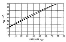
Figure 1. MPX12 Linearity Analysis Raw Data
