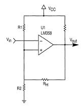
Figure 4. LM358 Comparator Circuit Schematic
