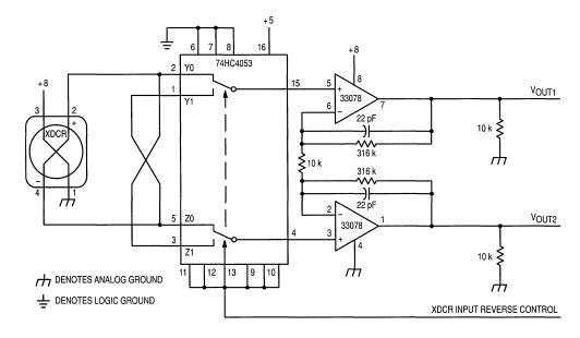
Figure 1. X-ducer, Instrument Amplifier and Analog Switch
