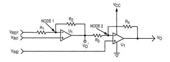
Figure 2. The Two Operational-Amplifier Gain Stage
