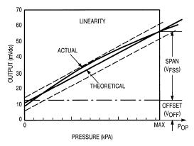
Figure 3. Linearity Specification Comparison
