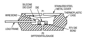
Figure 2. Cross-Sectional Diagrams (Not to Scale)
