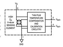
Figure 1. Temperature Compensated Pressure Sensor Schematic
