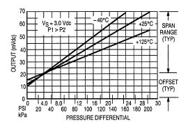
Figure 3. Output versus Pressure Differential
