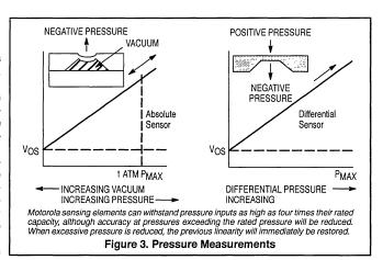
Gauge Pressure readings are a special case of differential measurements in which the pressure applied to the Pressure side is measured against the ambient atmospheric pressure applied to the Vacuum side through the vent
