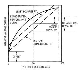
Figure 2. Linearity Specification Comparison
