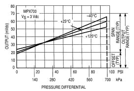
Figure 2. Output versus Pressure Differential
