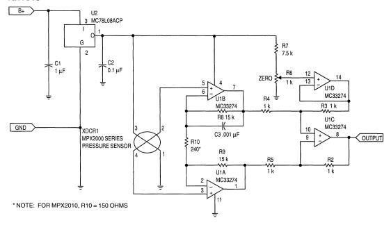
Figure 2. Instrumentation Amplifier Interface
