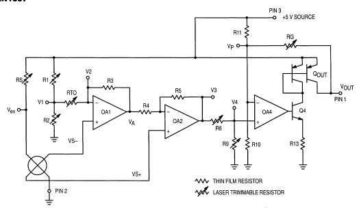
Figure 4. Fully Integrated Pressure Sensor Schematic
