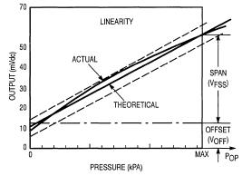
Figure 3. Linearity Specification Comparison
