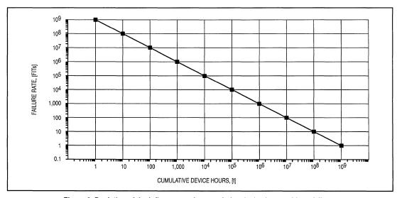
Figure 9. Depiction of the influence on the cumulative device hours with no failures and the Failure Rate as measured in FITs.
