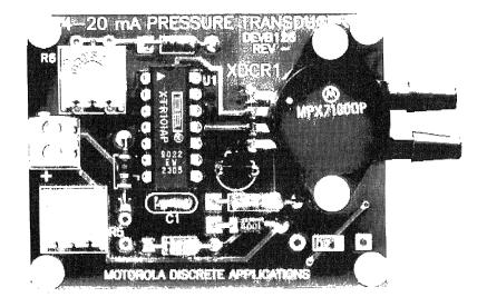
Figure 1. 4-20 mA Pressure Transducer Evaluation Board
