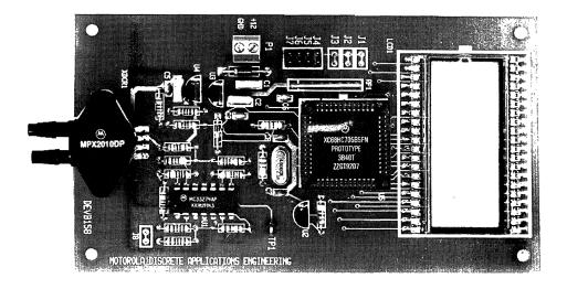
Figure 1. DEVB158 2000 Series LCD Pressure Gauge EVB
