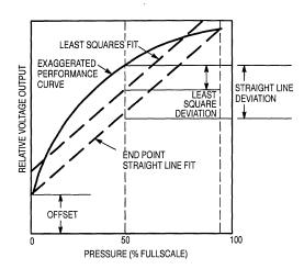
Figure 2. Linearity Specification Comparison
