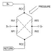
Figure 1. Sensor Equivalent Circuit
