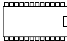
24-Pin SOIC Area = 165 mm 2
