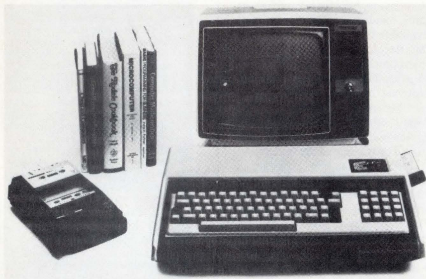
Fig 5 The exidy Sorcerer computer with a ROM-PACK plugged into the side. (Courtesy of Exidy, Data Products Div., Sunnyvale, CA)
