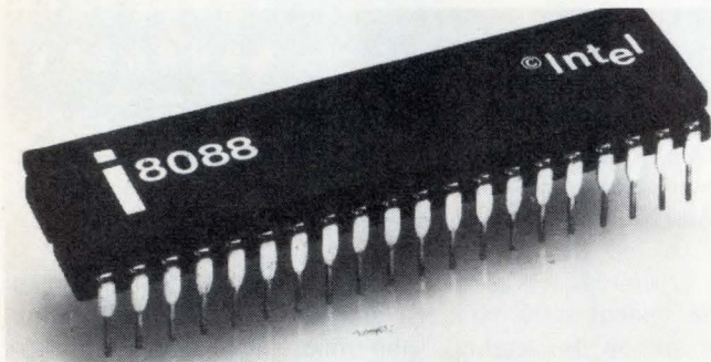
Intel's new 8088 contains the 16-bit internal architecture of the 8086 combined with the 8-bit bus interface of the 8085A to give it performance surpassing other current 8-bit devices.
