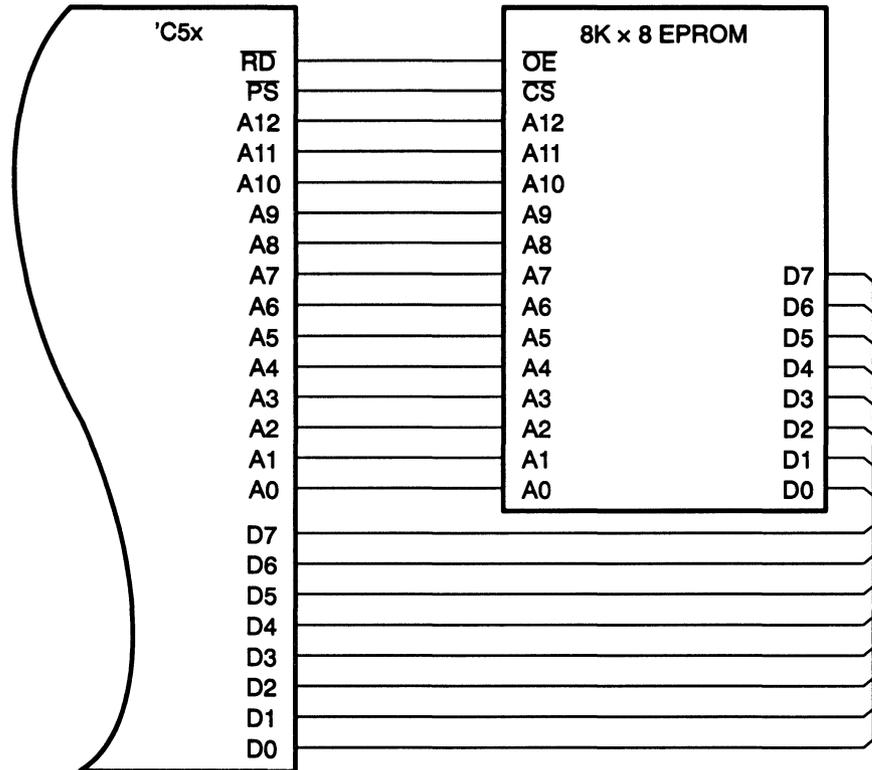
The program select ( $\overline{PS}$ ) signal is connected directly to the chip select ( $\overline{CS}$ ) to select the EPROM on any external program access. The EPROM is addressed in any 8K address block in program space. If multiple blocks of memory are to be interfaced in program space, a decode circuit that gates  $\overline{PS}$  and the appropriate address bits can be used to drive the memory block chip selects.
