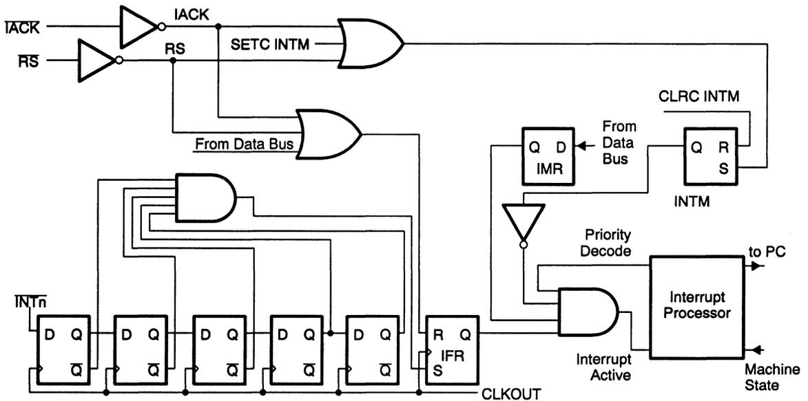
If the INTM bit and mask registers have been properly enabled, the interrupt signal is accepted by the processor. An IACK signal is then generated. The IACK clears the appropriate interrupt edge flip-flop and sets the INTM = 1. The logic is the same for INT1–INT4. NMI uses the same logic, except that it is not affected by IMR or INTM status.
