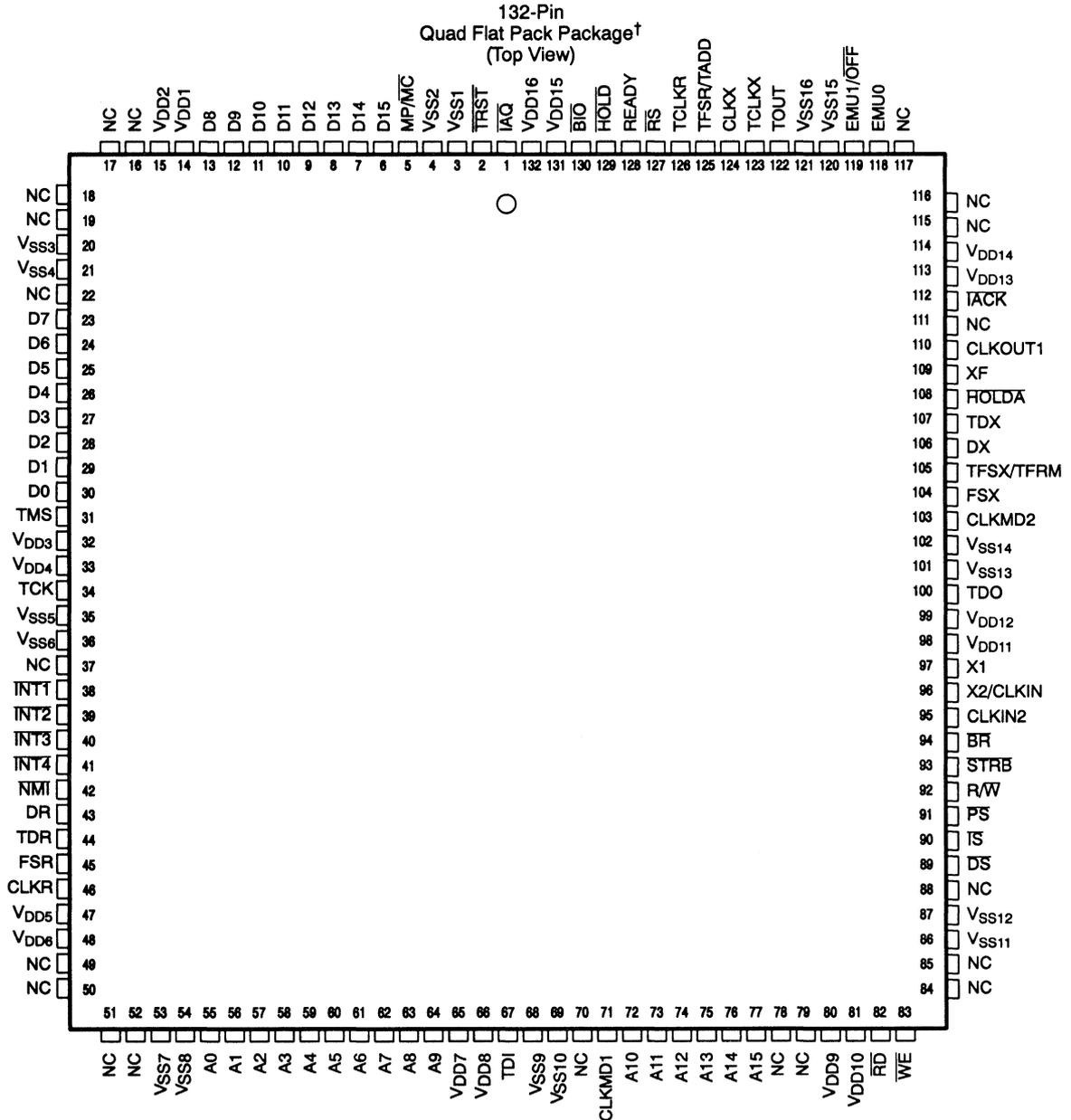
† See Pin Assignments, Table A–1 (page A-3) for location and description of all pins. The 'C50, 'C51, and 'C53 are packaged in 132-pin plastic QFP in production. See Figure A–20 for mechanical data.
