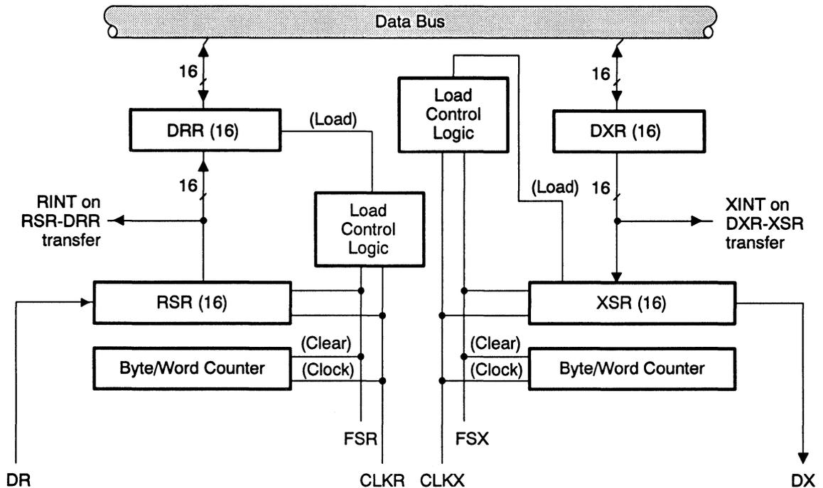
The SPC controls serial port operation; the functions of SPC bit fields are described in Table 5–8. Transmit data is written to the DXR, while received data is read from the DRR. A transmit is executed by writing data to the DXR, which copies the data to the XSR when the XSR is empty (the last word has been serially transmitted, that is, driven on the DX pin). The XSR manages the shifting of the data to the DX pin, thus allowing another write to DXR as soon as the DXR-to-XSR copy is completed.
