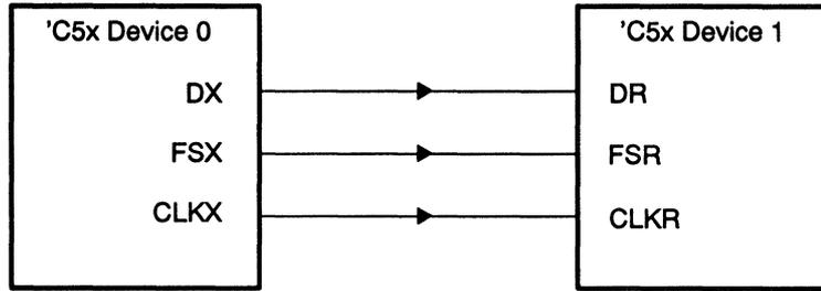
The serial port operates through the three memory-mapped registers (SPC, DXR, and DRR) and two other registers (XSR and RSR) that are not accessible but permit double-buffering capability. These five registers are listed in Table 5–7.
