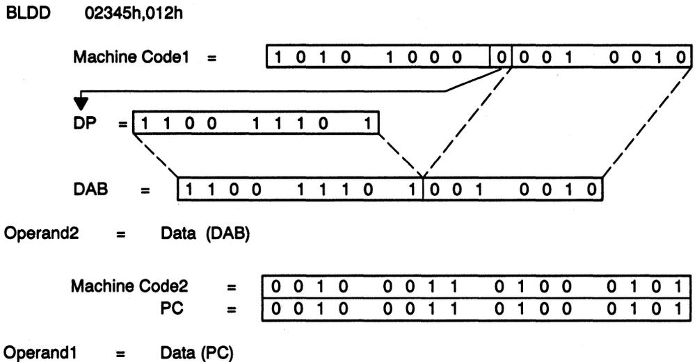
The registered block memory addressing mode operates like the long immediate addressing mode with the exception that the address comes from the BMAR register. The advantage of this technique over long immediate addressing is that it allows the address of the block of memory to be changed in run-time. On the other hand, the address in long immediate addressing mode resides in the program flow and cannot be easily changed. Figure 6–9 shows an example of registered block memory addressing mode.
