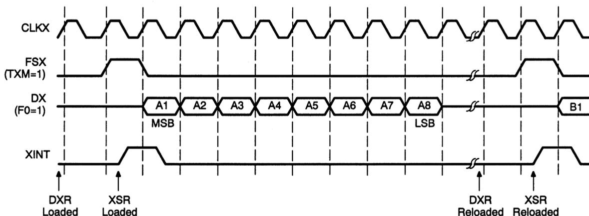
Note in the following discussion that the timings are slightly different for internally (TXM=1, FSX is an output) and externally (TXM=0, FSX is an input) gen-
