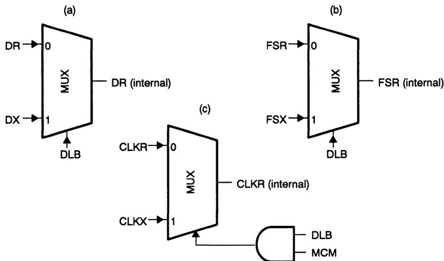
CLKR is driven by CLKX if MCM=1. But if MCM=0 while DLB=1, then CLKR is taken from the CLKR pin. This allows for external clock generation of these signals during digital loopback mode. If DLB=0, then normal operation occurs where DR, FSR, and CLKR are all taken from their respective pins.
