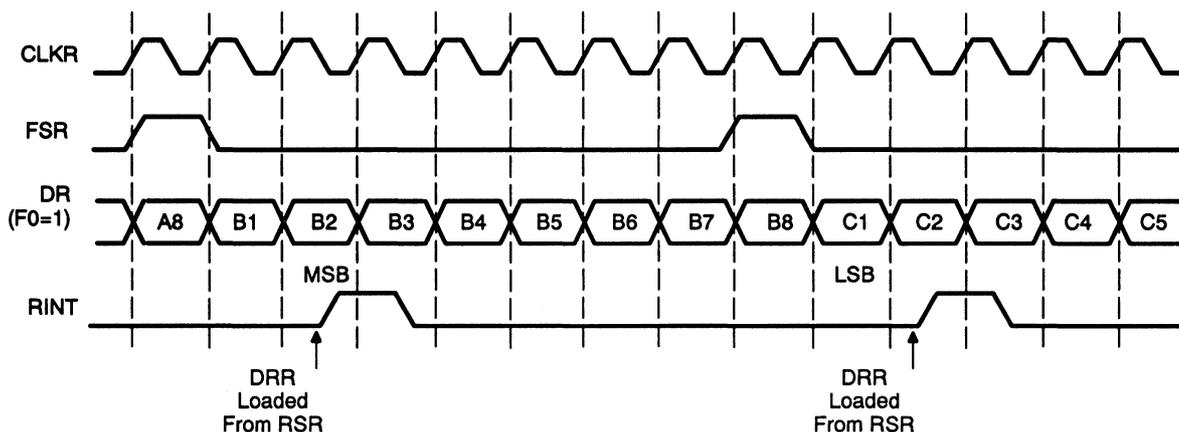
The maximum packet frequency transfer looks like a compressed version of burst mode with no periods of inactivity. The frame sync pulse overlaps the first bit transmitted.
