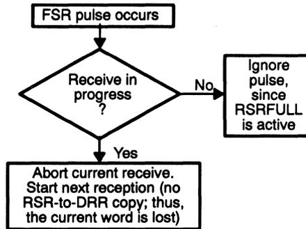
Figure 5–20. Transmit Error (Continuous Mode)
