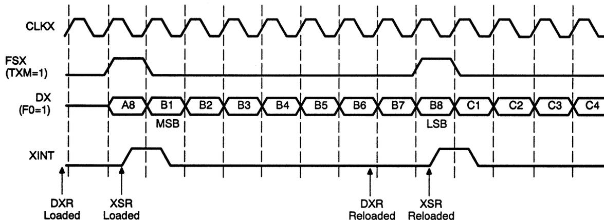
The data bits in consecutive packets are transmitted continuously with no inactivity in between the bits. The frame sync pulse overlaps the last bit transmitted in the previous packet. The receive side in Figure 5–13 looks similar.
