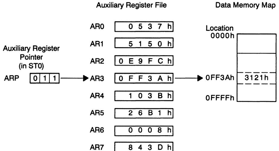
The auxiliary register file (AR0–AR7) is connected to the auxiliary register arithmetic unit (ARAU), shown in Figure 3–11. The ARAU may autoindex the current auxiliary register while the data memory location is being addressed. Indexing either by  $\pm 1$  or by the contents of the INDX register may be performed. As a result, accessing tables of information does not require the central arithmetic logic unit (CALU) for address manipulation; thus, the CALU is free for other operations in parallel.
