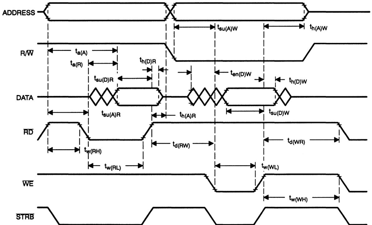
**Note:** All timings are for 0 wait states. However, external writes always require two cycles to prevent external bus conflicts. The above diagram illustrates a one-cycle read and a two-cycle write and is not drawn to scale. All external writes immediately preceded by an external read or immediately followed by an external read require three machine cycles.
