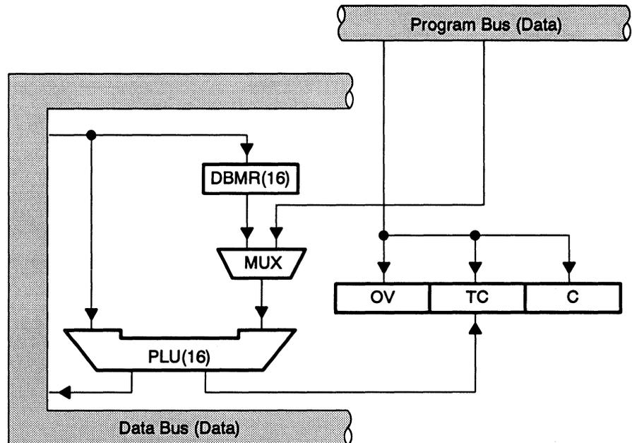
The PLU executes a read-modify-write operation on data stored in data space. The PLU operation begins with the fetching of one operand from data memory space and the fetching of the second from either long immediate on the program bus or the dynamic bit manipulation register (DBMR). Then, the PLU executes a logical operation defined by the instruction on the two operands. The result is written to the same data memory location from which the first operand was fetched.
