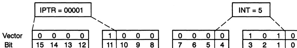
Upon reset, the IPTR bits are all set to zero, thus mapping the vectors to page zero in program memory space. This means the reset vector always resides at zero. The interrupt vectors can be moved to another location by loading a nonzero value into the IPTR bits. For example, the interrupt vectors can be moved to start at location 0800h by loading the IPTR with 1.
