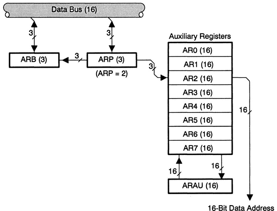
The contents of the auxiliary registers may be operated upon by the auxiliary register arithmetic unit (ARAU), which implements unsigned 16-bit arithmetic. The ARAU performs auxiliary register arithmetic operations in the decode phase of the pipeline. This allows the address to be generated before the decode phase of the next instruction. The AR is incremented or decremented after it is used in the current instruction.
