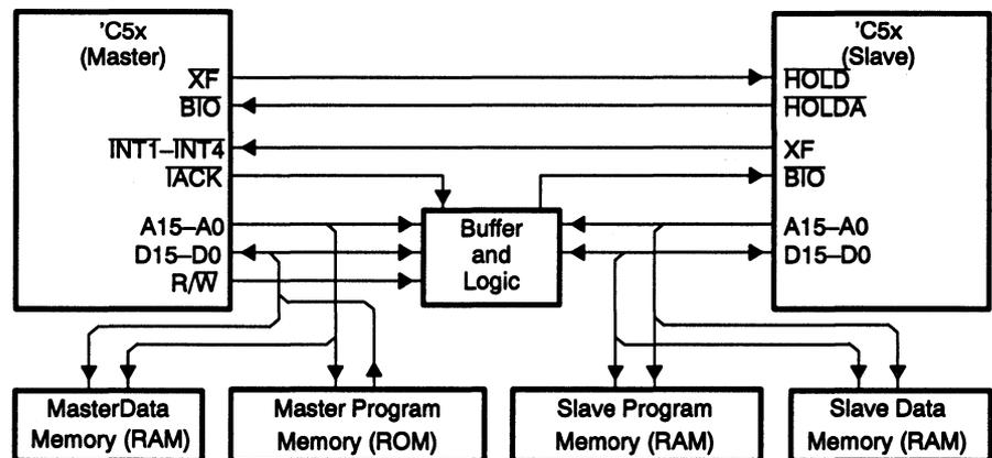
The master 'C5x device takes complete control of the slave's external memory by asserting  $\overline{\text{HOLD}}$  low via its external flag (XF). This causes the slave to place its address, data, and control lines in a high-impedance state.
