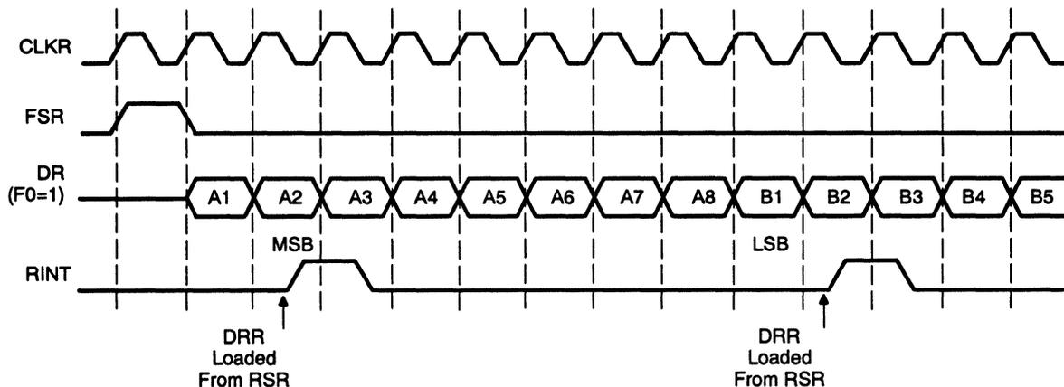
Figure 5–16 shows no frame signals; otherwise, it is similar to Figure 5–13. If a pulse occurs on FSR during transmission (an error), then the receive operation is aborted, one packet is lost, and a new receive cycle is begun. This is discussed in more detail on page 5-22.
