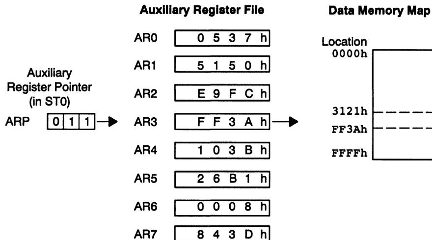
The auxiliary registers and the ARP can be updated directly from data memory, the accumulator, or the product register, or by an immediate operand defined in the instruction. The contents of these registers can also be stored in data memory or used as inputs to the CALU. These registers appear in the memory map as described in Table 6–8.
