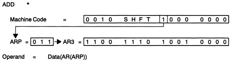
The operand may reside as part of the instruction machine code. In the case of the short immediate operand, the operand is contained in the single-word instruction. These short immediate operands vary in length from 1 bit on the SETC instruction to 13 bits on the MPY instruction. Figure 3–5 shows an example of short immediate mode. Note that, in this example, the lower eight bits are the operand and will be added to the ACC by the CALU.
