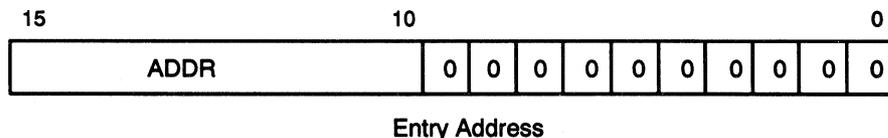
The 'C50 transfers control to the entry address if a warm boot is specified.
