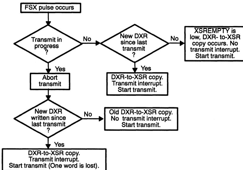
In continuous mode, errors take on a broader meaning. Data transfer is supposed to be occurring at all times in continuous mode. Thus, underflow
