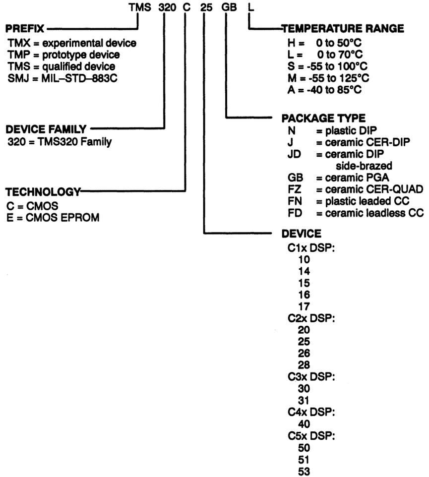
Figure I-2 provides a legend for reading the part number for any TMS320 hardware or software development tool.
