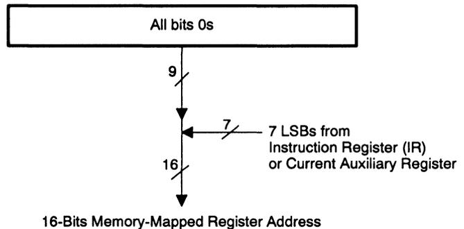
This addressing mode allows greater flexibility for dealing with memory-mapped registers. The overhead required to perform operations involving a memory-mapped register is greatly reduced because the data page pointer (DP) does not need to be modified before and after the operation. The following instructions operate in the memory-mapped register addressing mode:
