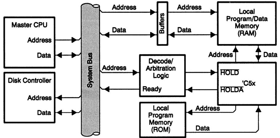
The 'C5x also provides direct access of the on-chip single-access RAM for external devices. DMA of the on-chip single-access RAM requires the following signals:
