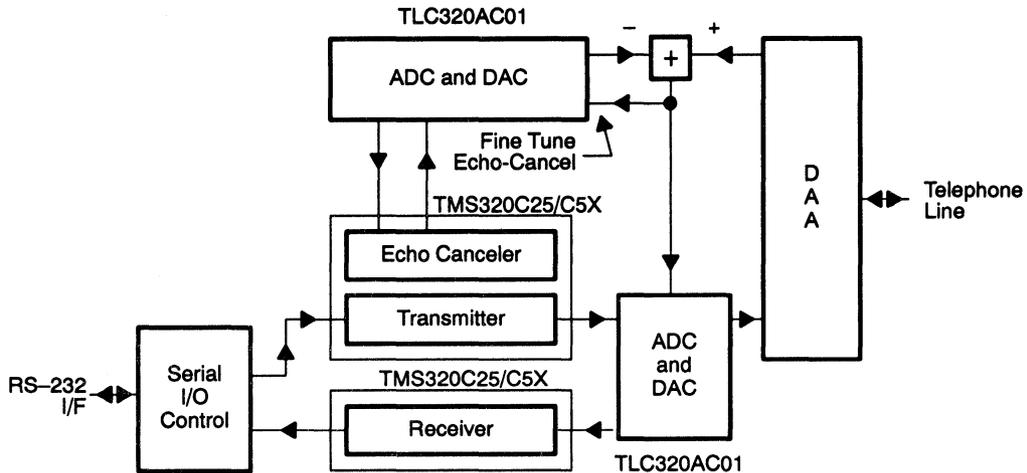
Figure F-11 shows a V.32 bis modem implementation using the 'C25 and a TLC320AC01. The upper 'C25 performs echo cancellation and transmit data functions, while the lower 'C25 performs receive data and timing recovery functions. The echo canceler simulates the telephone channel and generates an estimated echo of the transmit data signal. The TLC320AC01 performs the following functions:
