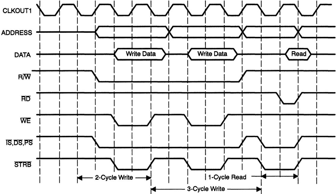
Figure B-3. Memory Interface Operation for Read-Write (1 Wait State)
