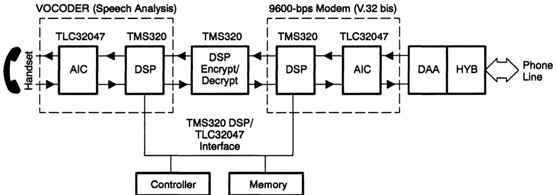
Figure F-3 shows the interfacing of the 'C25 DSP to the TLC32047 AIC that constitutes the building blocks of the 9600-bps V.32 bis modem shown in Figure F-2.
