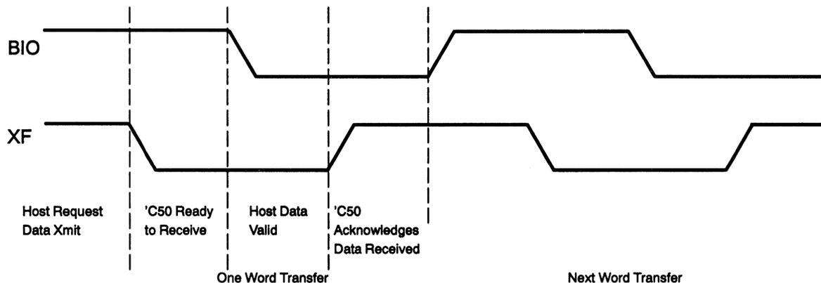
If the 8-bit transfer mode is selected, the lower eight data lines are read from port 50h. The upper byte on the data bus is ignored. The 'C50 reads two 8-bit words to form a 16-bit word. The low byte of a 16-bit word should follow the high byte.
