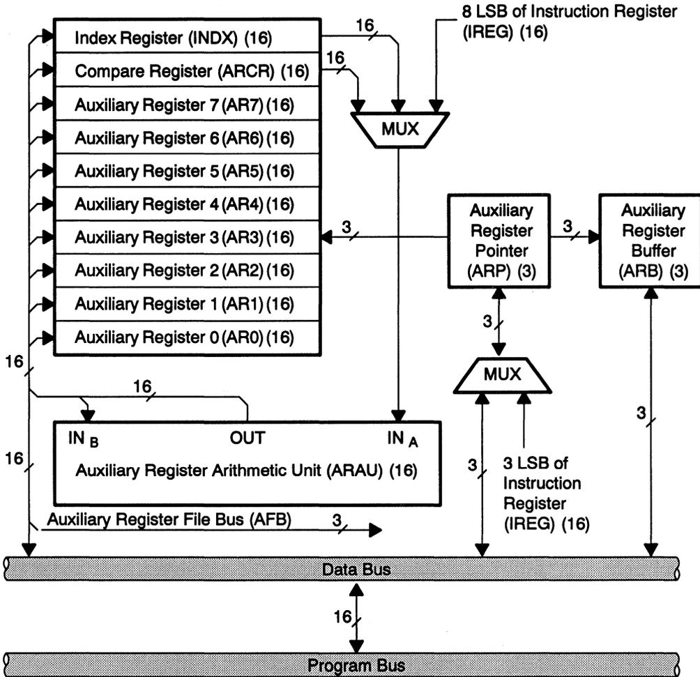
As shown in Figure 3–11, the index register, compare register, or the eight LSBs of the instruction register can be used as one of the inputs of the ARAU. The other input is fed by the current AR (being pointed to by ARP). AR(ARP) refers to the contents of the current AR pointed to by ARP. The ARAU performs the functions shown in Table 3–3.
