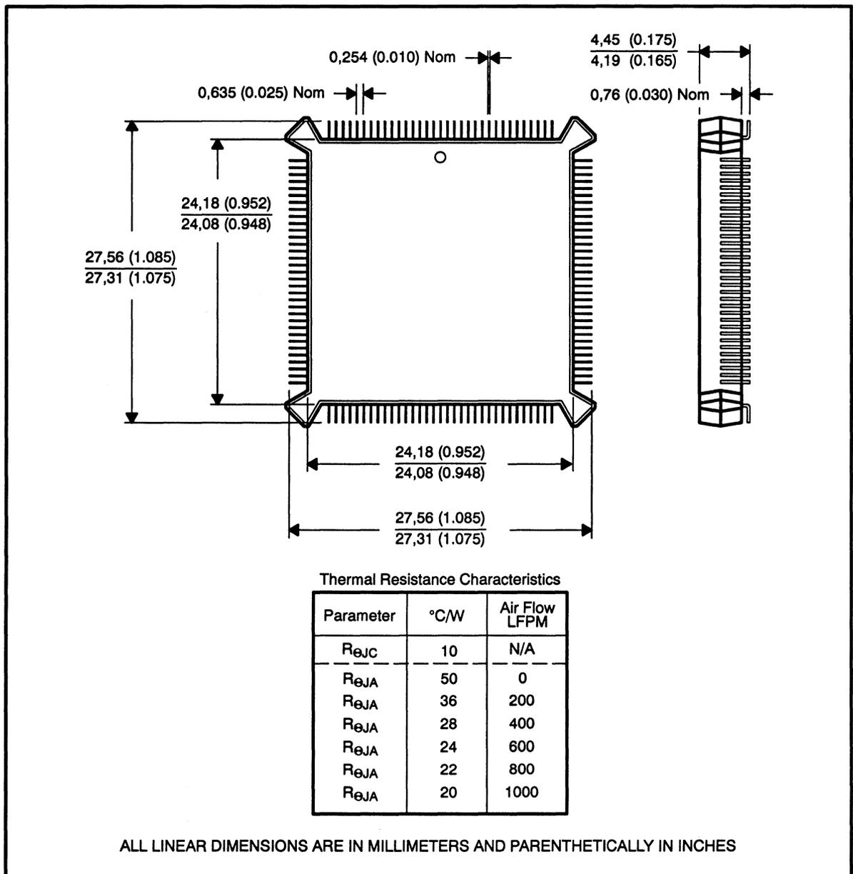
**Note:** The contact points are within 0,15 (0.006) of being planar.
