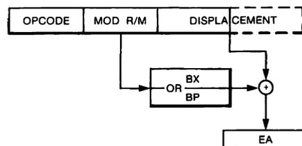
**Figure 28: Accessing a Structure with Based Addressing**
