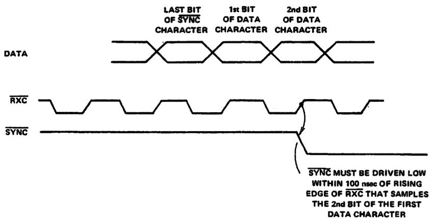
**Figure G-2.4 SYNC Output, Internal Synchronization**
