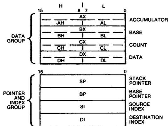
The data registers are unique in that their upper (high) and lower halves are separately addressable. Each data register can be used interchangeably as a 16-bit register or as two 8-bit registers. However, the CPU registers are always accessed as 16-bit units. Data registers can be used without constraint in most arithmetic and logic operations. Certain instructions use specified registers implicitly (see Table 1), allowing compact, powerful encoding.
