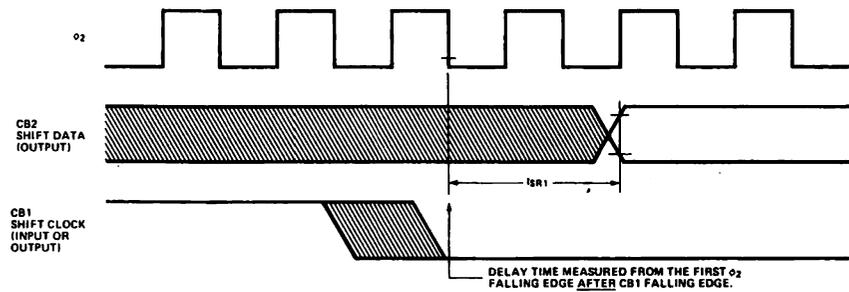
**Figure H-5g: Timing for Shift In with Internal or External Shift Clocking**
