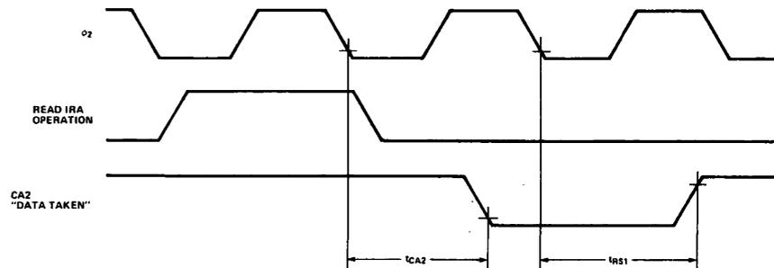
**Figure H-5b: CA2 Timing for Read Handshake, Handshake Mode**
