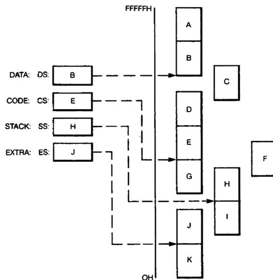
Individual applications define and use segments differently. The currently-addressable segments provide a generous work space: 64K bytes for code, a 64K byte stack, and 128K bytes of data storage. Many applications can be written that simply initialize the segment registers and then forget them. However, large applications should be designed with careful consideration given to segment definition.
