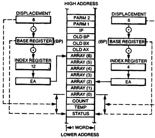
**STRING ADDRESSING** String instructions do not use the normal memory addressing modes to access their operands. Instead, the index registers are used implicitly as shown in Figure 33. When a string instruction is executed, SI is assumed to point to the first byte or word of the source string, and DI is assumed to point to the first byte or word of the destination string. In a repeated string operation, the CPUs automatically adjust SI and DI to obtain subsequent bytes or words.
