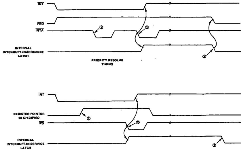
At the beginning of the first Interrupt Acknowledge cycle, the interrupt prioritization logic is frozen to permit any late interrupt requests by higher priority devices to ripple through and resolve internal priorities before the second interrupt pulse.
