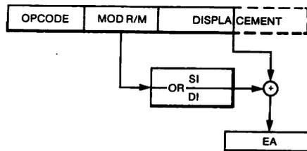
**Figure 30: Accessing an Array with Indexed Addressing**
