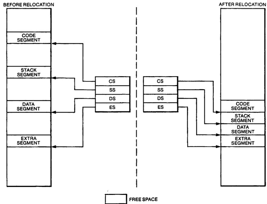
To be dynamically relocatable, all offsets in the program must be relative to fixed values contained in the segment registers. This allows the program to be moved anywhere in memory as long as the segment registers are updated to point to the new base addresses. A dynamically relocatable program must not load or alter its segment registers and must not transfer directly to a location outside the current code segment.
