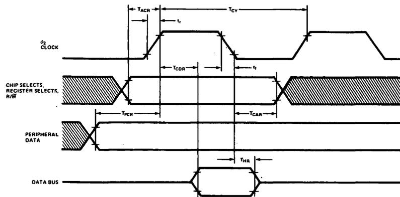
**READ TIMING CHARACTERISTICS (FIGURE H-3)**
