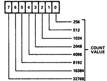
**WRITE** – 8 BITS LOADED INTO T1 HIGH-ORDER LATCHES. UNLIKE REG 4 OPERATION NO LATCH-TO-COUNTER TRANSFERS TAKE PLACE.
