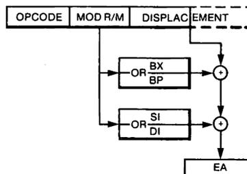
**Figure 32: Addressing a Stack Array with Based Indexed Addressing**
