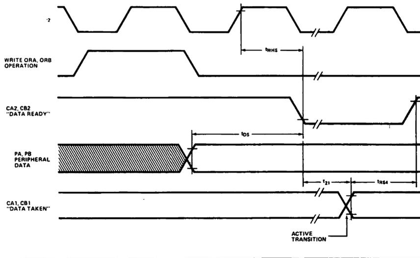
**Figure H-5e: Peripheral Data Input Latching Timing**
