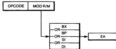
NOTE: Any 16-bit general register can be used for register indirect addressing with the JMP or CALL instructions.
