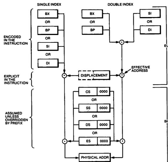
The displacement, an 8- or 16-bit number contained in the instruction, is derived from the position of the operand name (a variable or label) in the program. A programmer can modify this value or specify the displacement.
