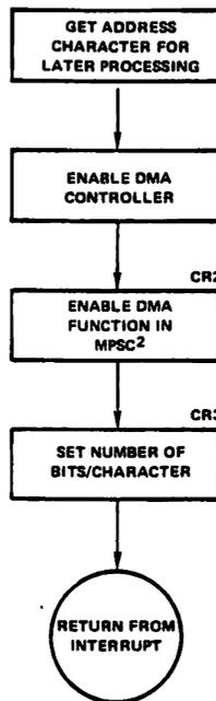
THE MPSC<sup>2</sup> IS NOW IN THE ADDRESS SEARCH PHASE. DURING THIS PHASE THE MPSC<sup>2</sup> INTERRUPTS WHEN THE PROGRAMMED ADDRESS MATCHES THE MESSAGE.
