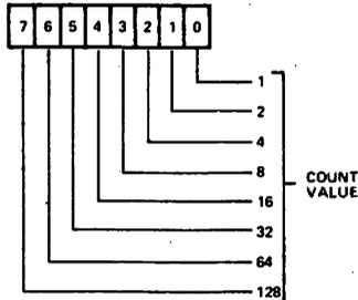
**WRITE** – 8 BITS LOADED INTO T1 LOW-ORDER LATCHES. THIS OPERATION IS NO DIFFERENT THAN A WRITE INTO REG 4.
