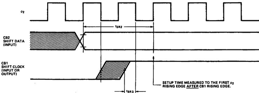
**Figure H-5h: External Shift Clock Timing**
