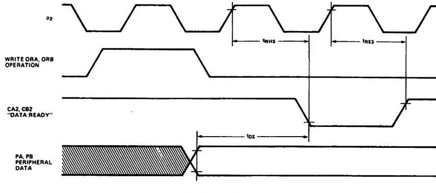
**Figure H-5d: CA2, CB2 Timing for Write Handshake, Handshake Mode**
