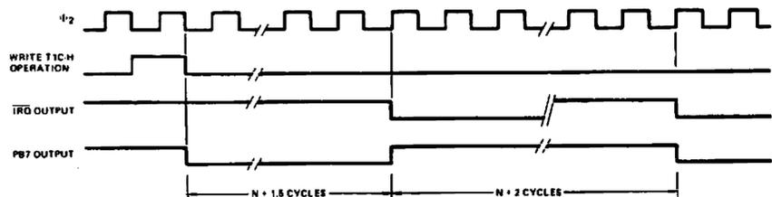
Note: A precaution to take in the use of PB7 as the timer output concerns the Data Direction Register contents for PB7. Both DDRB bit 7 and ACR bit 7 must be 1 for PB7 to function as the timer output. If one is 1 and the other is 0, then PB7 functions as a normal output pin, controlled by ORB bit 7.
