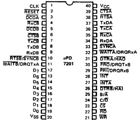
**12-19 D<sub>0</sub>-D<sub>7</sub> Data Bus (bidirectional three-state)**
