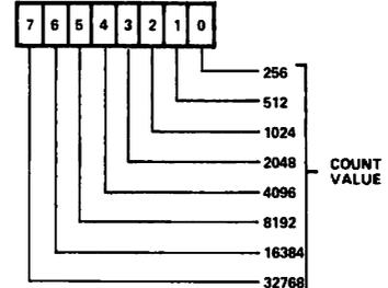
**WRITE** – 8 BITS LOADED INTO T1 HIGH-ORDER LATCHES. ALSO, AT THIS TIME BOTH HIGH AND LOW-ORDER LATCHES TRANSFERRED INTO T1 COUNTER. T1 INTERRUPT FLAG ALSO IS RESET.
