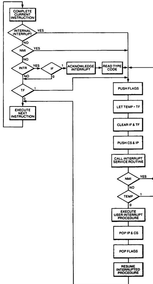
**EXTERNAL INTERRUPTS** External devices can use two lines in the 8088 to signal interrupts: interrupt request (INTR) and nonmaskable interrupt (NMI). The INTR line is driven by an 8259A programmable interrupt controller (PIC). The PIC is a flexible circuit controlled by software commands from the 8088.
