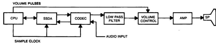
The synchronous serial data adapter (SSDA) is the major interface between the CPU and the audio section. The main function of the SSDA in playback mode is the buffering and conversion of 8-bit bytes into a serial bit stream for the Codec. In the record mode, the SSDA also converts a serial bit stream from the Codec into bytes for the CPU.
