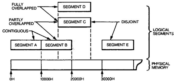
The segment registers contain (point to) the base address values of the four currently addressable segments (see Figure 14). Programs access code and data in other segments by changing the segment registers to point to the segments containing the needed code or data.
