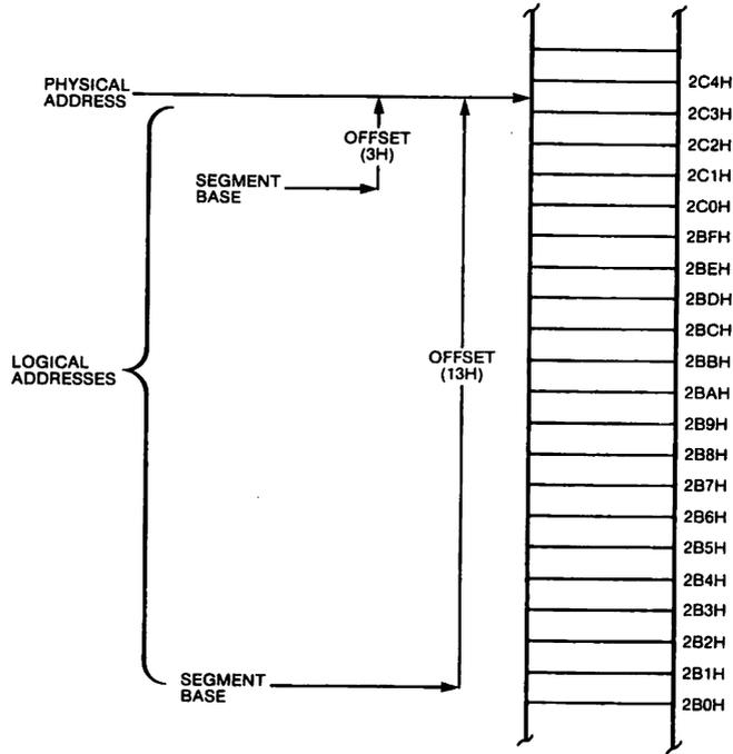
When the BIU accesses memory to fetch an instruction, or to obtain or store a variable, it generates a physical address from a logical address. It does this by (1) shifting the segment-base value four bit positions, and (2) adding the offset value, as illustrated in Figure 16. This addition process results in modulo 64K addressing, which causes addresses to wrap around from the end of a segment to the beginning of the same segment.
