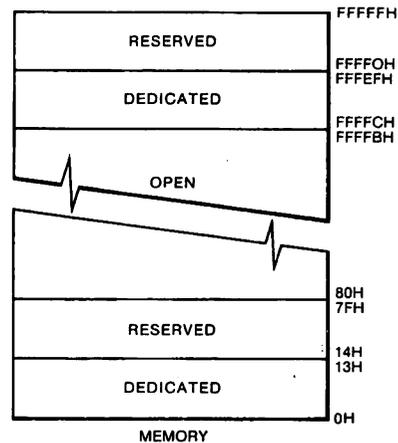
**8086/8088 MEMORY ACCESS** The 8088 always accesses memory in bytes. Word operands are accessed in two bus cycles, regardless of their alignment. Instructions are also fetched one byte at a time. Although word operand alignment does not affect performance, locating 16-bit data on even addresses ensures maximum throughput if the system is transferred to an 8086.
