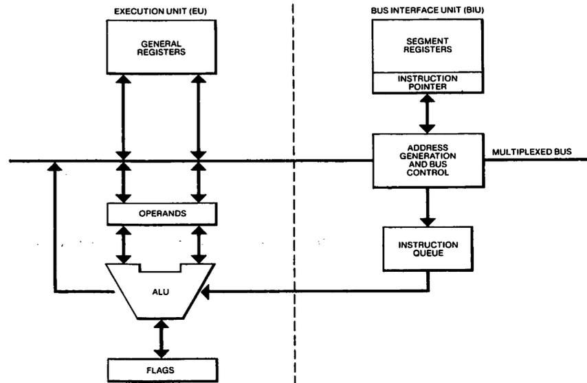
The EU is not connected to the outside world via the system bus. It obtains instructions from a queue maintained by the BIU. When an instruction requires access to memory or to a peripheral device, the EU sends a request to the BIU to store or obtain the data. The BIU performs an address relocation that gives the EU access to a full megabyte of memory space.
