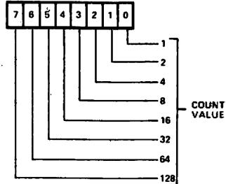
**WRITE** – 8 BITS LOADED INTO T1 LOW-ORDER LATCHES. LATCH CONTENTS ARE TRANSFERRED INTO LOW-ORDER COUNTER AT THE TIME THE HIGH-ORDER COUNTER IS LOADED (REG 5).
