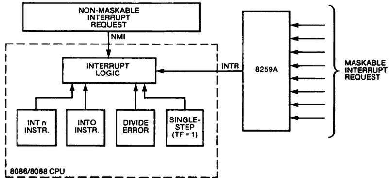
**Figure 21: Interrupt Processing Sequence**
