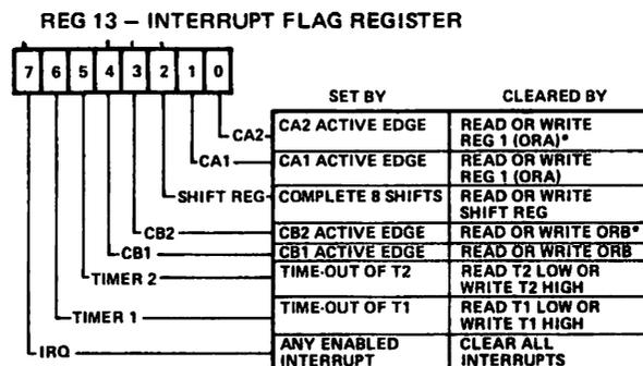
\* IF THE CA2/CB2 CONTROL IN THE PCR IS SELECTED AS "INDEPENDENT" INTERRUPT INPUT, THEN READING OR WRITING THE OUTPUT REGISTER ORA/ORB WILL NOT CLEAR THE FLAG BIT. INSTEAD, THE BIT MUST BE CLEARED BY WRITING INTO THE IFR, AS DESCRIBED PREVIOUSLY.
