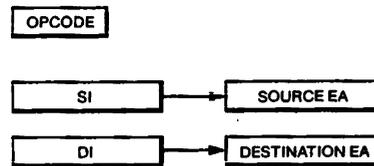
**I/O PORT ADDRESSING** When an I/O port is memory mapped, any of the memory operand addressing modes can be used to access the port. For example, a group of terminals can be accessed as an array. String instructions can also transfer data to memory-mapped ports with an appropriate hardware interface.
